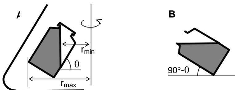
**Fig. 4. Liquid surface during rotation (A) and calculation of safe amount of liquid (B).**
