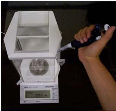
**Fig. 7 Calibration of Pipetman**
