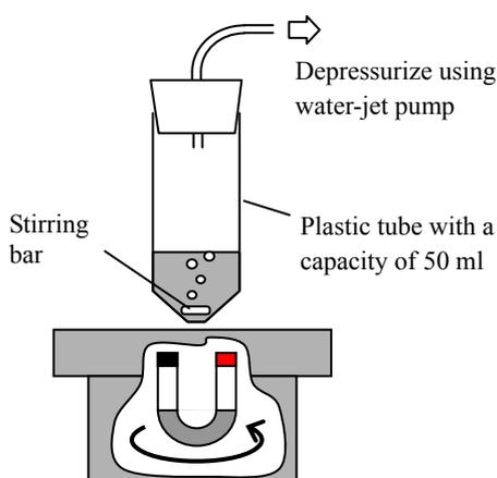
**Fig. 13 Degassing of gel solution**
