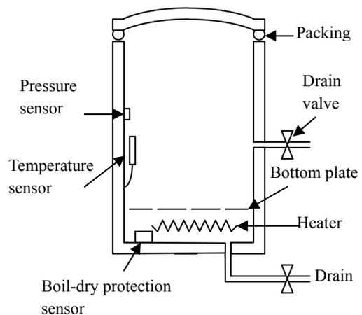
**Fig. 1 Structure of autoclave**
