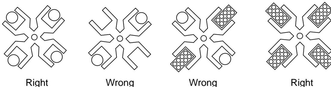
**Fig. 6 Right and wrong mounting of assemblies for swing-type centrifuge**
