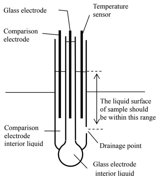
**Fig. 10 Structure of pH Sensor**
