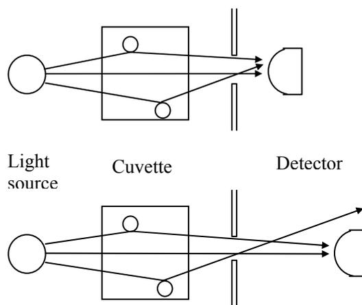
**Fig. 11 Effect of detector position on turbidity measurement.**
